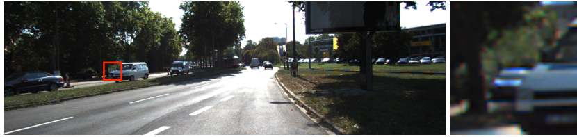
Figure 9: Failure case of the inferred 3D rigid motion model. The small blue car is partially occluded by the white van in the first frame, and is completely invisible in the second. The estimated visual cues are thus completely wrong (unlike background it cannot benefit from other observations). It leads to 5 m translation error and 17.5 degree angular error.
