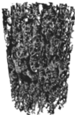
micro-CT @ 22 \mu\text{m} resolution ( 8 \text{ mm} H: 15 \text{ mm} D)
