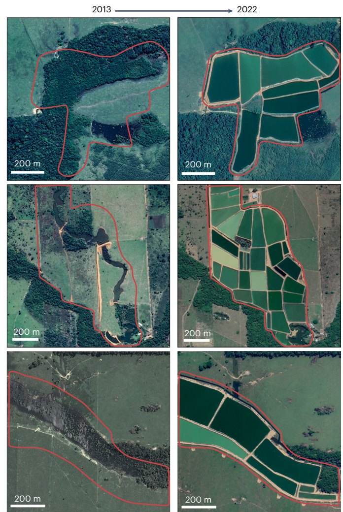
Fig. 4 | Satellite images from 2013 and 2022 from three sites with constructed fish ponds in Rondônia reveal myriad land-use transitions associated with expanding aquaculture, which need to be integrated into land-use and GHG accounting. Left: 2013; right: 2022. The red lines circle the same area in both years for reference to the previous land cover. Credit: satellite photographs, Google, ©2024 Maxar Technologies, CNES/Airbus.
