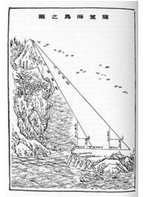
Liu Hui (c. 263), How to measure the height of a sea island.
