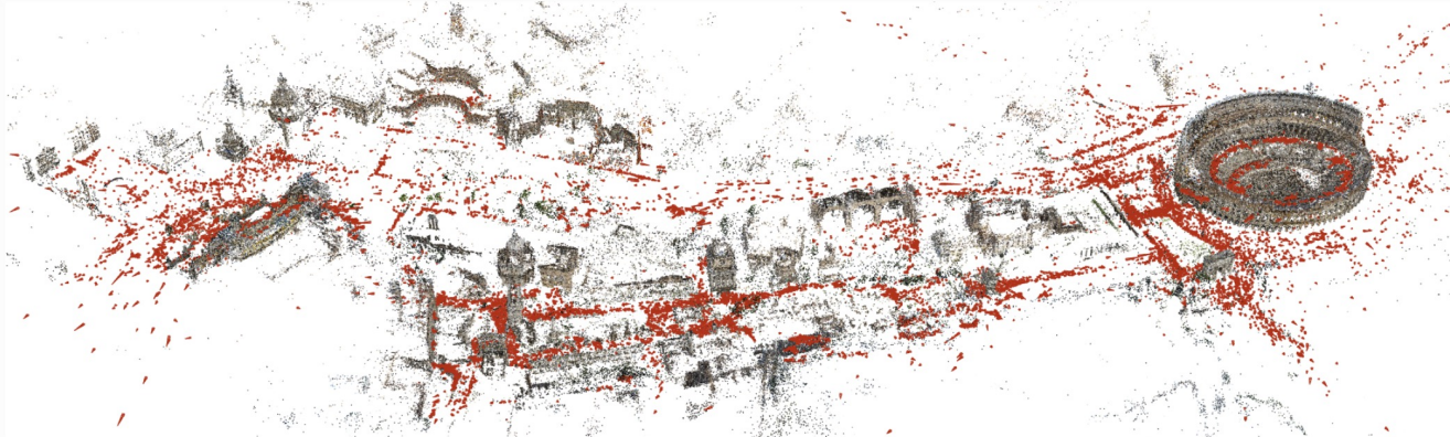
Sparse model of central Rome using 21K photos produced by COLMAP's SfM pipeline.
