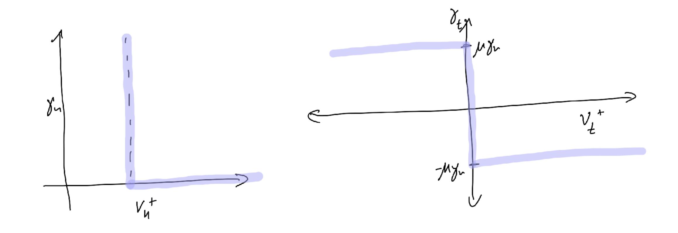
Start with relative velocity but keep normal and tangential components
