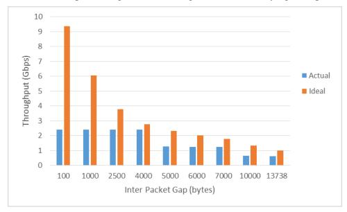
We got maximum throughput of 2.42 Gbps with inter packet gap of 100 bytes. We also measured throughput with different Ethernet frame sizes keeping inter packet gap 13738 bytes and got the following results:
