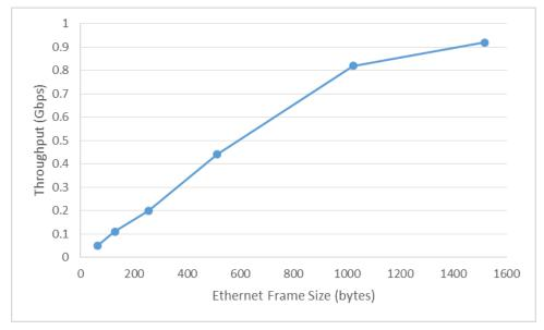
We got maximum throughput of 0.92 Gbps with Ethernet frame size of 1518 bytes. We also made our implementation work across SoNIC cards and got the following results while varying inter packet gap:
