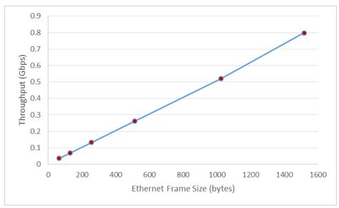
Throughput increases by increasing Ethernet frame size as increasing frame size results in more bandwidth utilization for sending data. We got maximum throughput of 0.79 Gbps with frame size of 1518 bytes.
