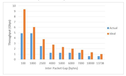
Throughput decreases as we increase the Inter Packet Gap because more and more channel bandwidth is consumed by idle packets. We got maximum throughput of 4.88 Gbps with inter packet gap of 100 bytes. We also measured throughput by varying Ethernet frame size and got the following results:
