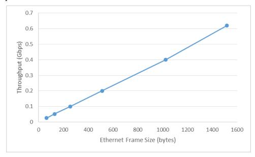
We got maximum throughput of 0.62 Gbps with Ethernet frame size of 1518 bytes.
