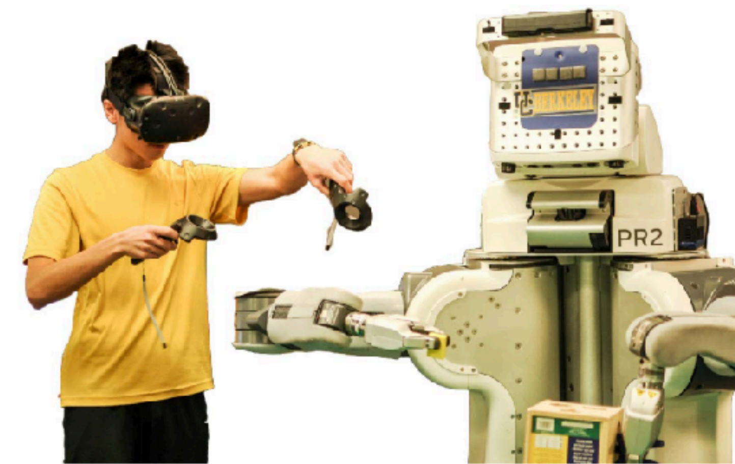
Fig. 1: Virtual Reality teleoperation in action
