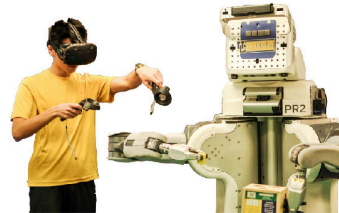
Fig. 1: Virtual Reality teleoperation in action
