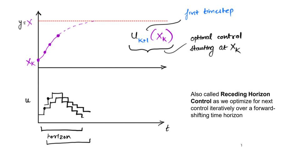
**Dynamics model / Process model**: Informs about the possible future states of the system as well as the constraints associated with it
