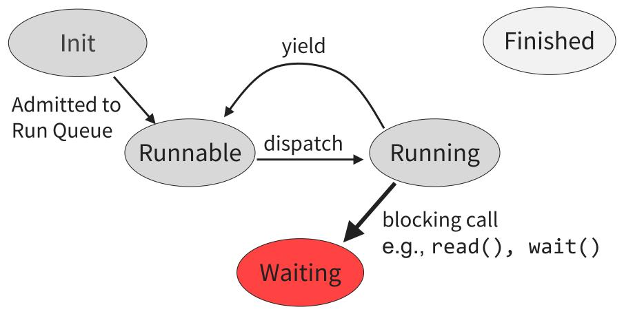
**PCB:** on specific waiting queue (file input, ...) **Registers:** on interrupt stack
