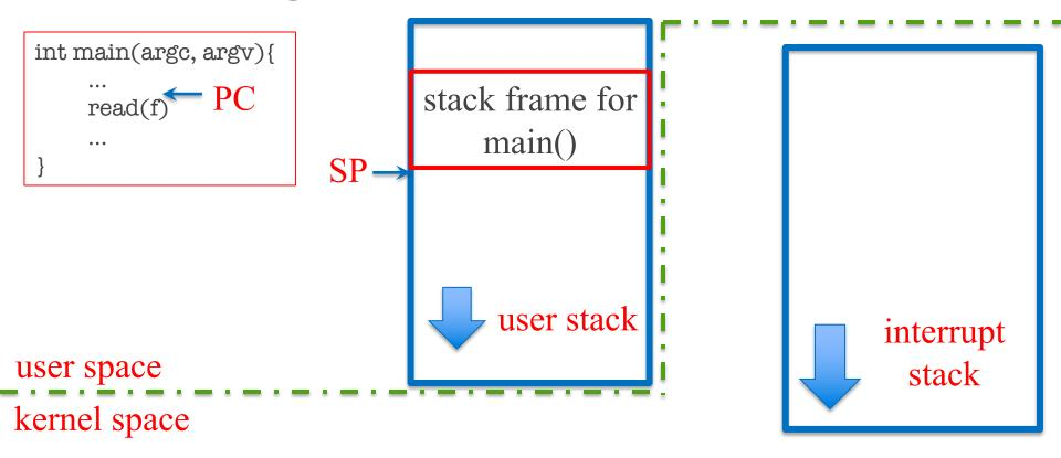
note interrupt stack empty while process running
