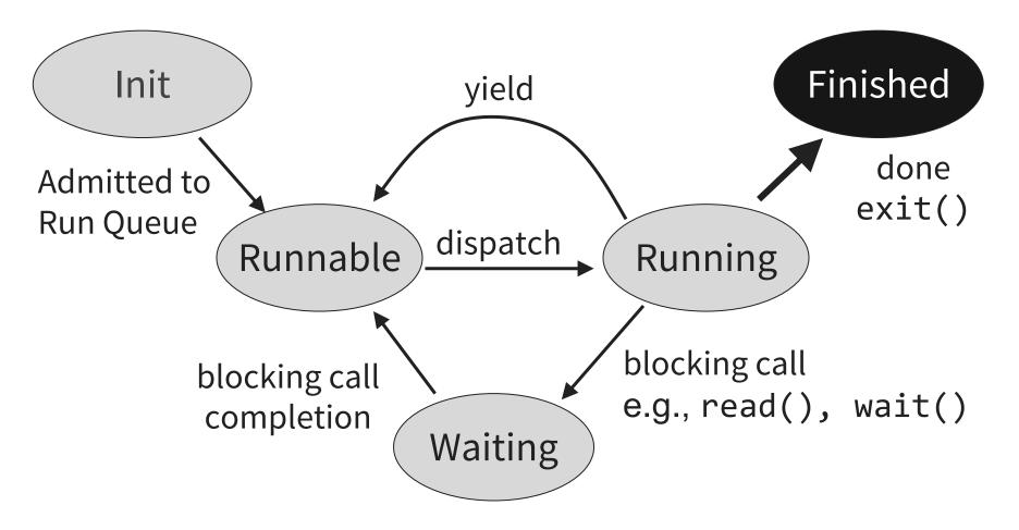
**PCB:** on Finished queue, ultimately deleted **Registers:** no longer needed
