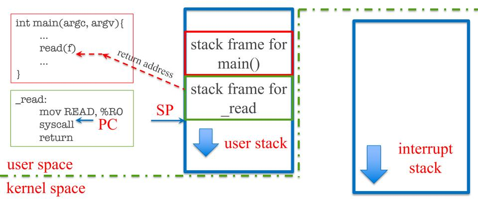
note interrupt stack empty while process running
