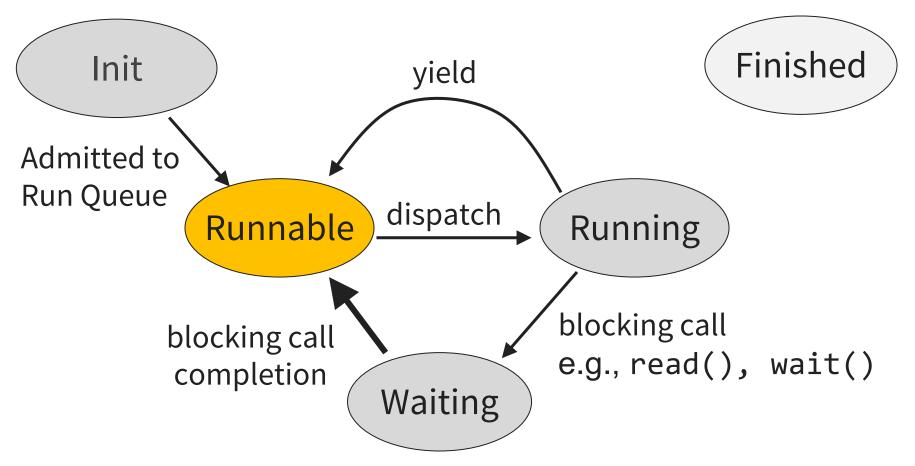
**PCB:** on run queue **Registers:** on interrupt stack
