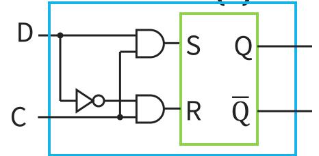
C = 1, D Latch *transparent*: set/reset (according to D) C = 0, D Latch *opaque*: keep state (ignore D)
