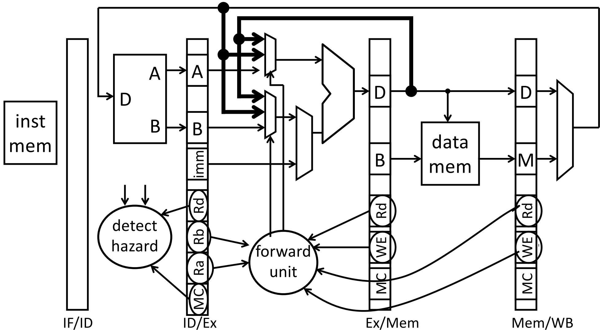
$\text{Stall} = \text{If}(\text{ID/Ex.MemRead} \And \text{IF/ID.Ra} == \text{ID/Ex.Rd})$
