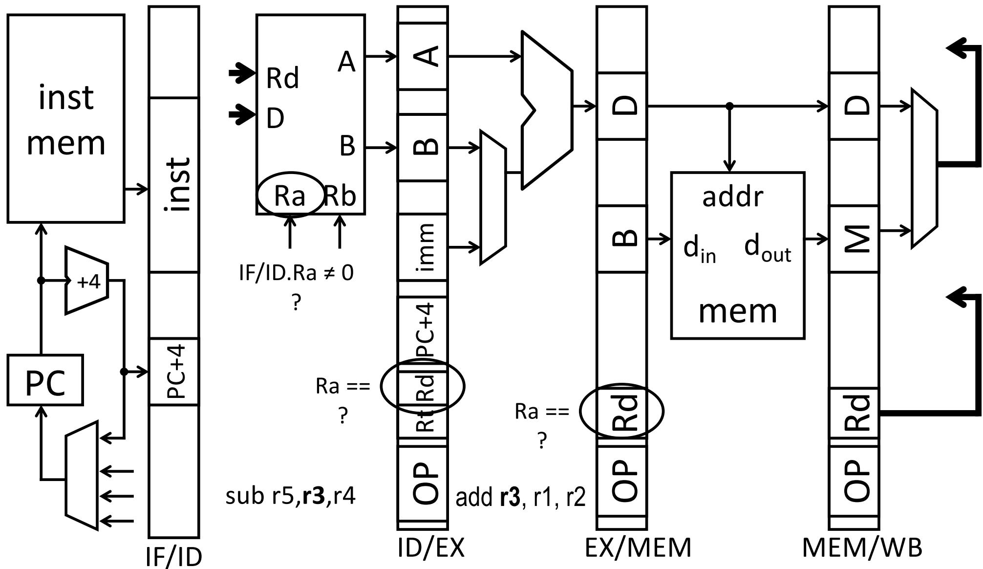
Problem =  $(\text{IF/ID.Ra} \neq 0 \ \&\& \ (\text{IF/ID.Ra} == \text{ID/EX.Rd} \ | \ | \ \text{IF/ID.Ra} == \text{EX/MEM.Rd}))$
