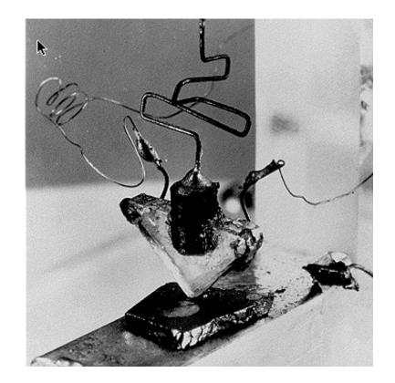
The first transistor on a workbench at AT&T Bell Labs in 1947
