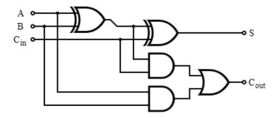
In the above diagram, A and B are the 1-bit inputs, while  $C_{in}$  is the carry-in bit. S is the output bit, while  $C_{out}$  is the carry-out bit. This is the optimal circuit for the following truth table:
