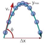
$$\begin{array}{rcl} v_x & = & dx/dt \\ v_y & = & dy/dt \\ dv_x/dt & = & -k \cdot v_x \sqrt{v_x^2 + v_y^2} \\ dv_y/dt & = & -k \cdot v_y \sqrt{v_x^2 + v_y^2} - g \end{array}$$
