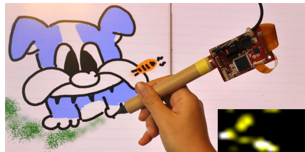
Figure 1. Our MTPen prototype. Inset image shows touch data imaged by the multi-touch sensor around the barrel.
