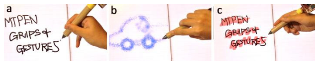
Figure 9. Pen selection based on grip: (a) Pen ink for the tripod grip, (b) paintbrush for the sketch grip, and (c) highlighter for the relaxed tripod grip.
