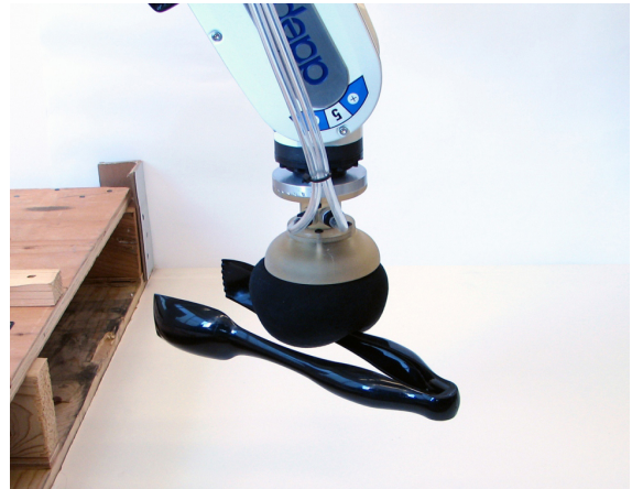
Fig. 1: The universal jamming gripper shown choosing a successful grasp point on a target object using our hardware agnostic learning algorithm.
