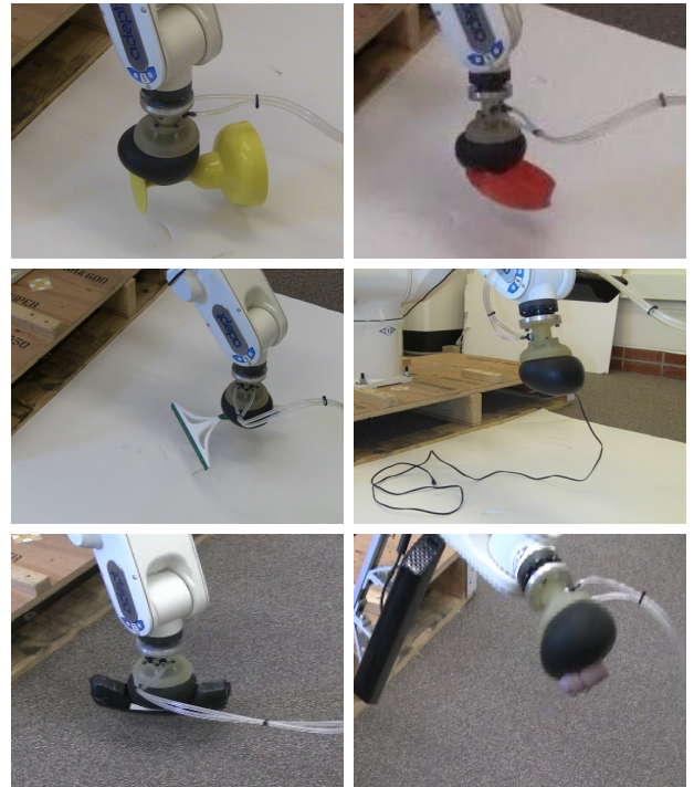
Fig. 4: The universal jamming gripper grasping different objects.
