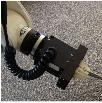
Fig. 5: The traditional two-jaw gripper that is used to compare with the universal jamming gripper.
