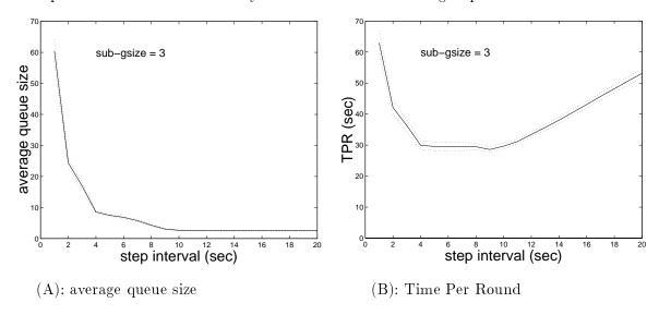
Figure 4: Simulation I (no message loss) with a dense group of size 200, and sub-group size 3.
