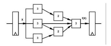
Blocks with a *vee* correspond to positive edge-triggered flip-flops. Assume, for simplicity, that flip-flops do not introduce any additional delay. You can only introduce flip-flops on the arrows shown in the figure.
