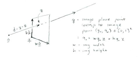
We can easily compute  $\mathbf{q}$  if we have a basis for the view rectangle. Let  $\mathbf{q}_0$  be the lower left corner of the image plane, and let  $\hat{\mathbf{u}}$  and  $\hat{\mathbf{v}}$  be the vectors along the bottom and left edges. Then if  $(q_u, q_v)$ are the coordinates of a point in the image, defined in the unit square:
