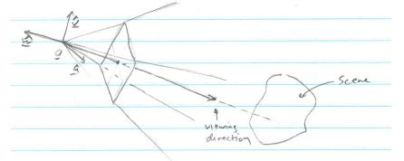
So for pose all we need to do is store the eye point and these three vectors. We can use them to find the image plane (by moving along  $-\hat{\mathbf{w}}$  from the eye point) and to move around on the image plane (by adding  $\hat{\mathbf{u}}$  and  $\hat{\mathbf{v}}$ ).
