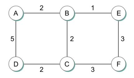
In the above network, links are labeled with costs. Assume we have distance-vector routing. Give the routing tables when
