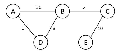
In the above network, links are labeled with costs. Assume we use the basic distance vector algorithm.
