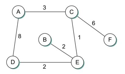
In the above network, links are labeled with costs. Assume distance vector routing.
