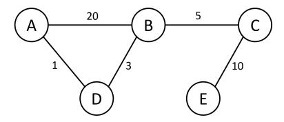
In the above network, links are labeled with costs. Assume we use the basic distance vector algorithm.
