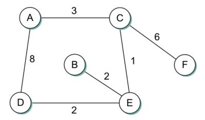
In the above network, links are labeled with costs. Assume distance-vector routing.
