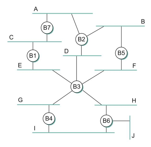
Above an extended LAN and its corresponding network graph is given.
